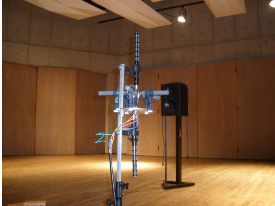
Figure 11: Spatial microphone array (height has been lowered for setup) with room excitation source (speaker) in background.
